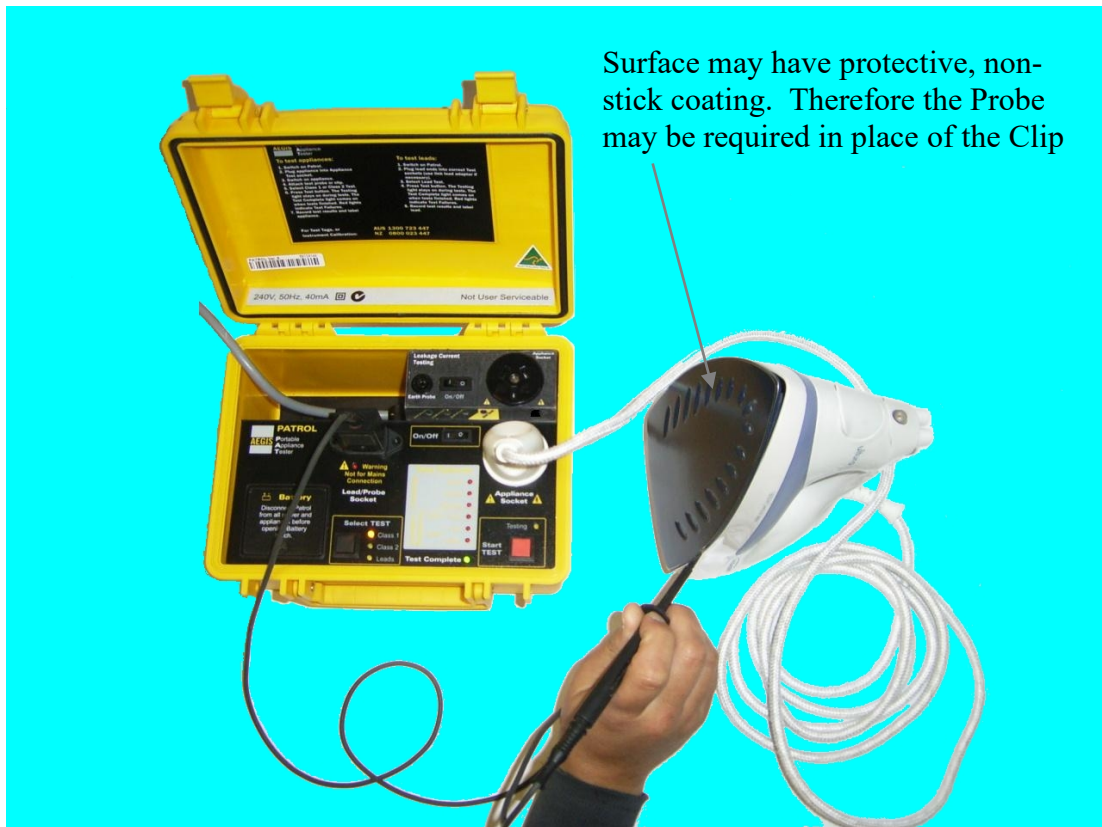
Figure 4.2.1-1 Class 1 Appliance Test connections.
