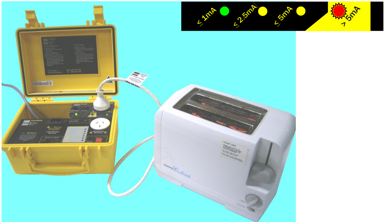
Figure 4.6-1 Class I Appliance Fail.
