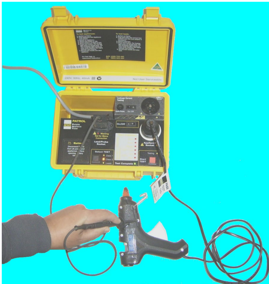
Figure 4.2.2-2 Class 2 Appliance Test Connection using the Probe
