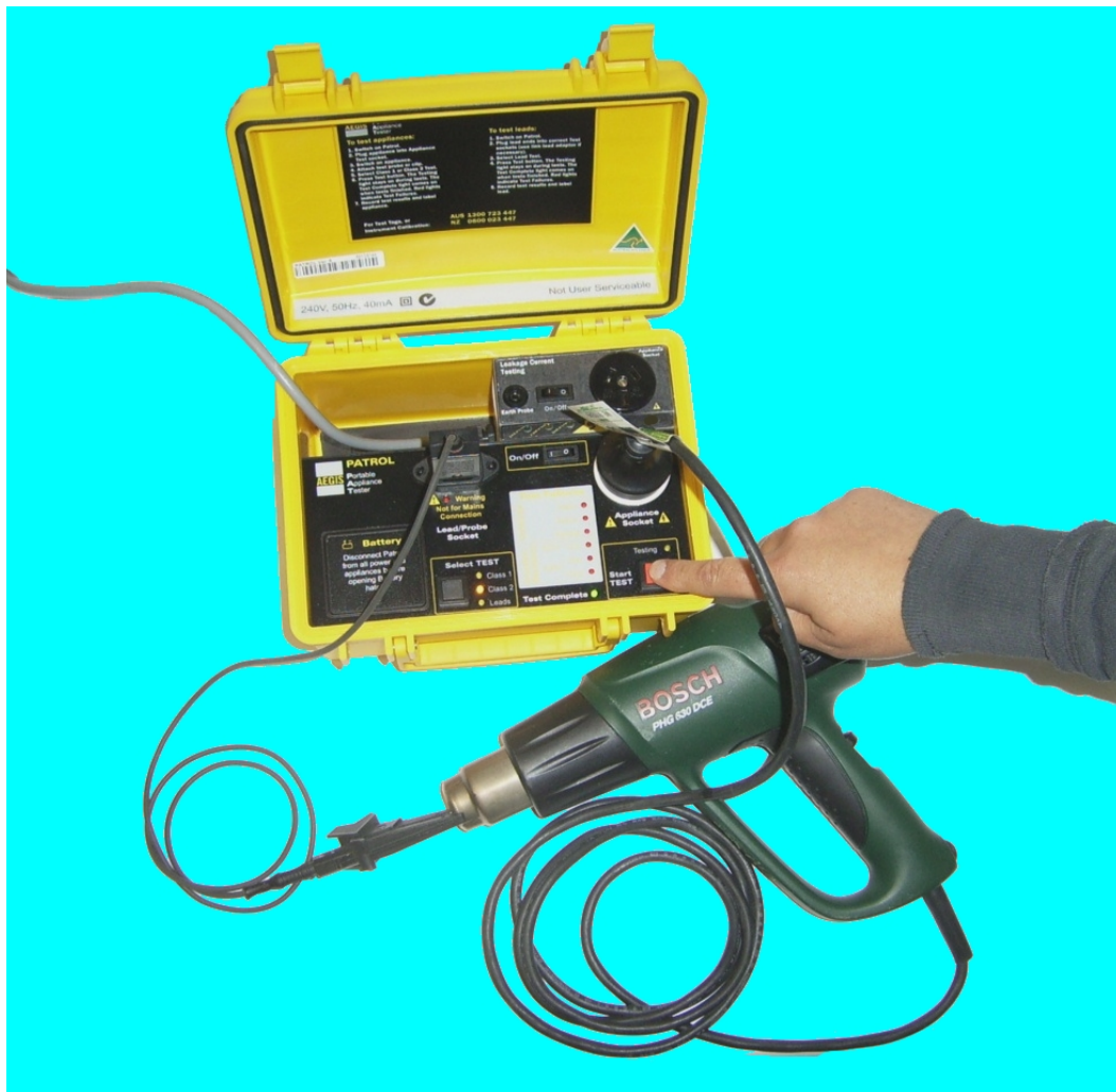
Figure 4.2.2-3 Class 2 Appliance Test Connection using the Clip
