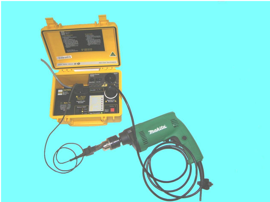
Figure 4.2.2-1 Class 2 Appliance Test connections, using the Clip
