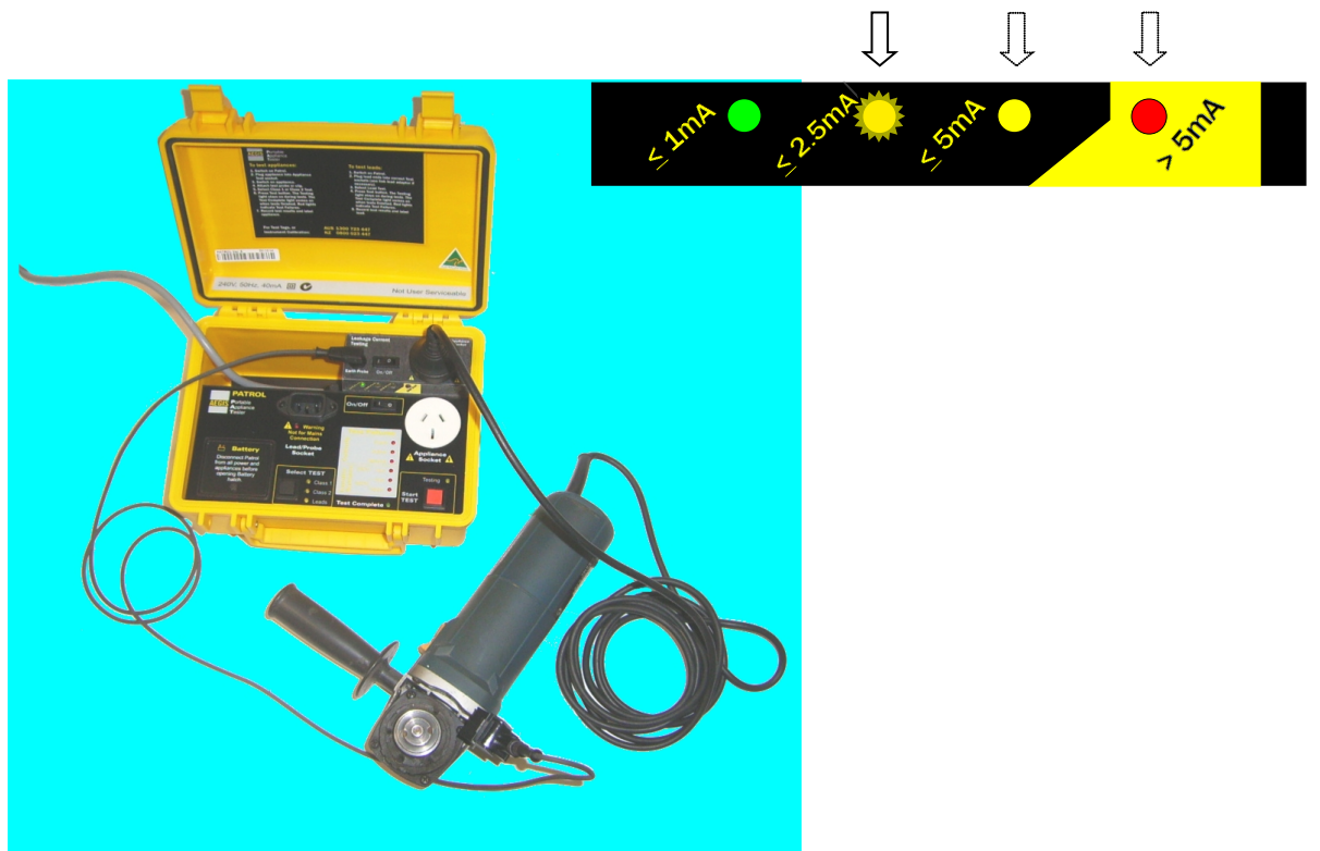
Figure 4.6-2 Class II Appliance Fail.
