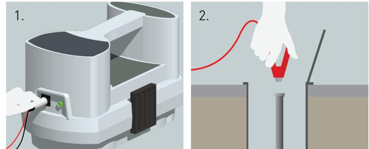
4. Place the Earth Stake in the ground (having first searched the area for buried cables with the Locator).
