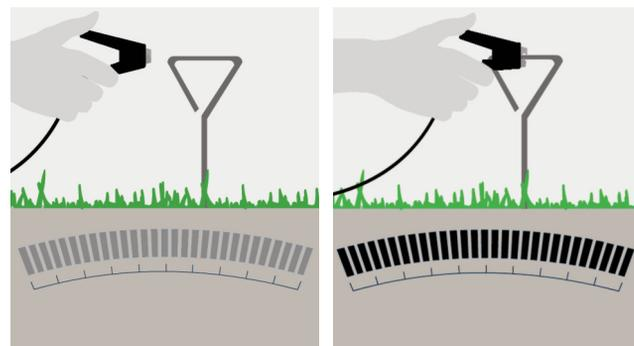
**i** **NOTE** If it is not possible to use the Earth Stake use a nearby metal fence post, manhole cover or gully cover. **DO NOT** use something that may have another metallic service attached to it, such as a metal street lighting column.
