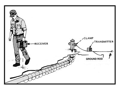
to cross back past the path of this conductor and will induce a certain amount of signal into it. This signal can mislead you when tracing it out.
